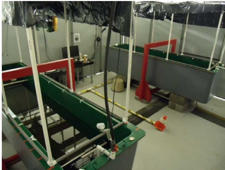
Figure 2.9. Control and EMF Exposure Tanks for Dungeness Crab Avoidance/Attraction Experiments
