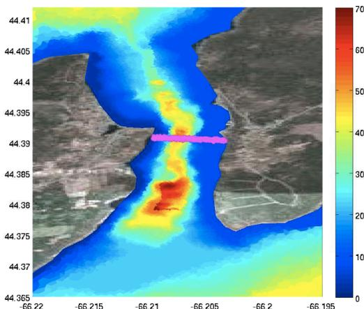
**Fig. 6:** The water depth (in metres) at mean tide in Petit Passage. The pink line is the location of the turbine fence.
