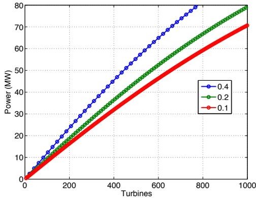
**Fig. 10:** Turbine power versus the number of turbines for Digby Gut, for the three different blockage ratios shown in the legend. Each dot represents an additional row of turbines.
