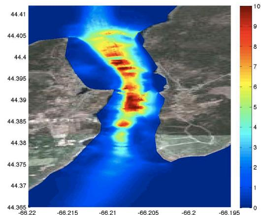
**Fig. 8:** The time-mean power density in kW/m<sup>2</sup> for Petit Passage.
