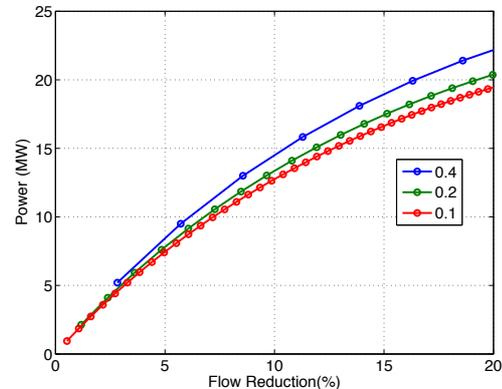
**Fig. 13:** Turbine power versus the flow reduction for Petit Passage, for the three different blockage ratios shown in the legend. Each dot represents an additional row of turbines.
