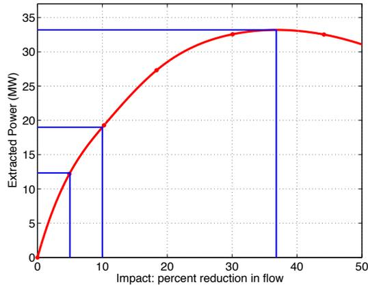
**Fig. 9:** Extracted power versus the reduction in flow through the turbine fence for Petit Passage. The blue lines highlight the values presented Table 1. The dots are the values for the individual simulations, the curve is found using an interpolating spline.
