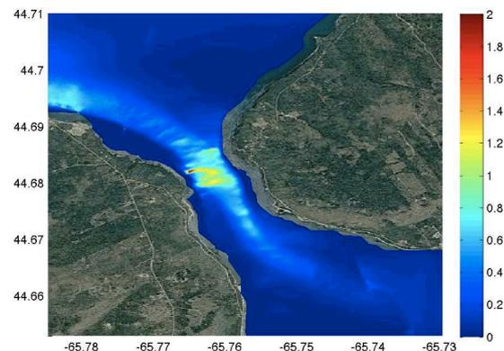
**Fig. 4:** The time-mean power density in kW/m<sup>2</sup> for Digby Gut.
