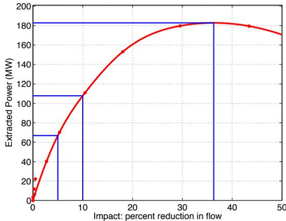
**Fig. 5:** Extracted power versus the reduction in flow through the turbine fence for Digby Gut. The blue lines highlight the values presented in Table 1. The dots are the values for the individual simulations.
