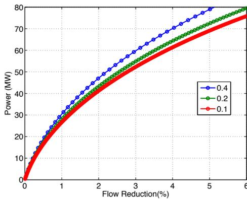
**Fig. 11:** Turbine power versus the flow reduction for Digby Gut, for the three different blockage ratios shown in the legend. Each dot represents an additional row of turbines.
