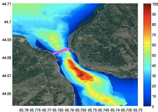
**Fig. 2:** The water depth (in metres) at mean tide in Digby Gut. The pink line is the location of the turbine fence.
