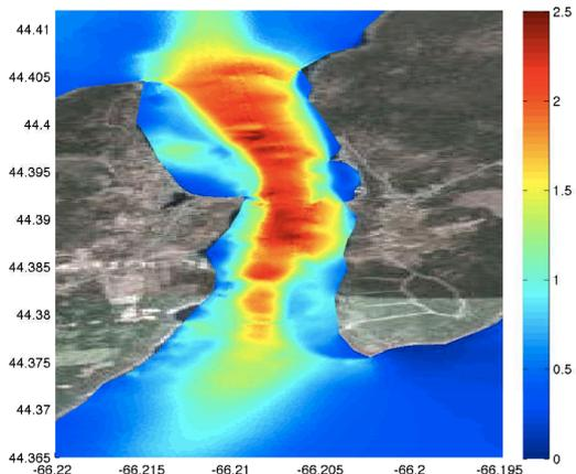
**Fig. 7:** The time-mean, depth-averaged speed in m/s for Petit Passage.
