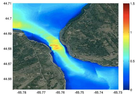
**Fig. 3:** The time-mean, depth-averaged speed in m/s for Digby Gut.
