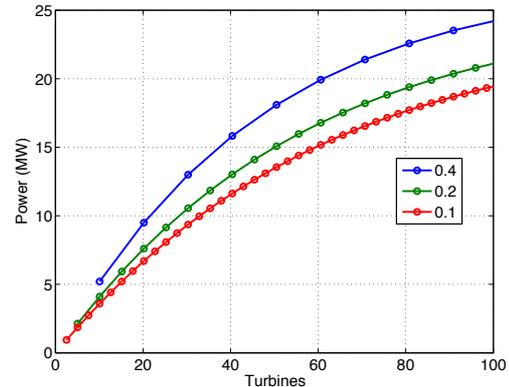
**Fig. 12:** Turbine power versus the number of turbines for Petit Passage, for the three different blockage ratios shown in the legend. Each dot represents an additional row of turbines.
