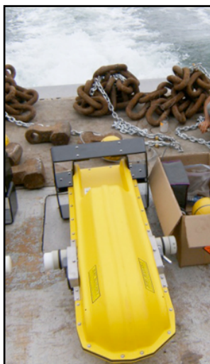
Figure 1: C-POD mounted in Sub-Buoy mooring - ready to deploy. Photo: Colin Buhariwalla.
