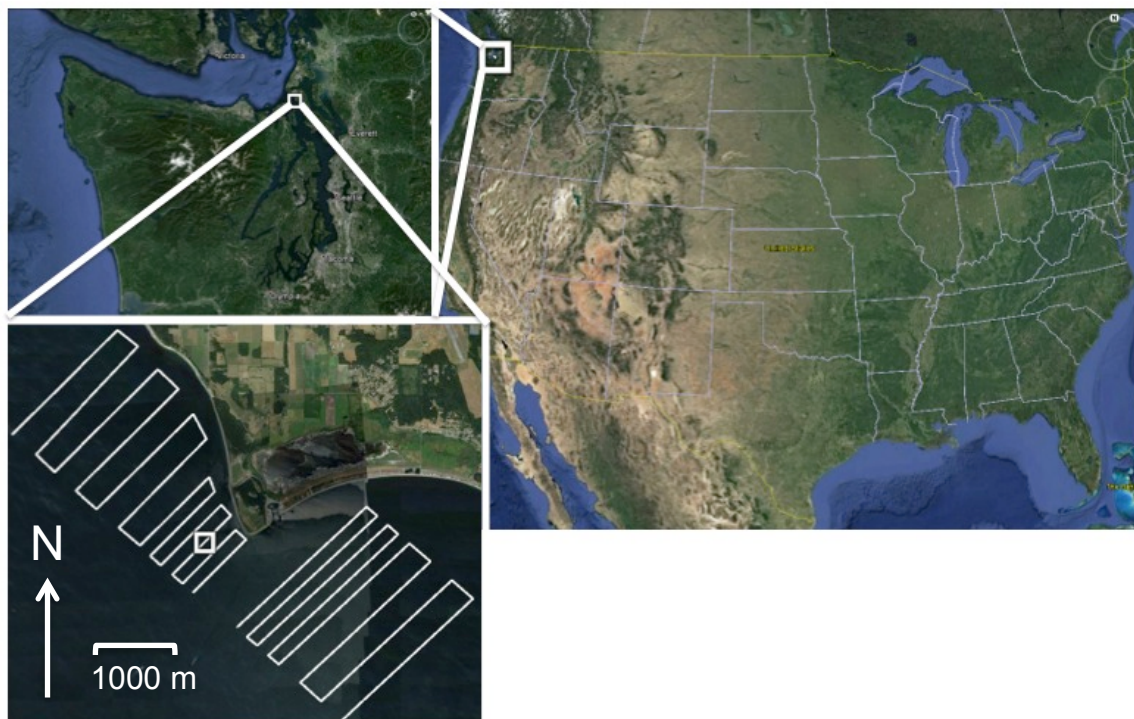
Figure 3.1. Admiralty Inlet, Puget Sound, USA. (top left) Admiralty Inlet at the mouth of Puget Sound. (bottom left) the location of the stationary echosounder, at a proposed tidal energy pilot site, is denoted by the white square in relation to the two spatial grids north and south of the stationary package, each consisting of high and low resolution transects.
