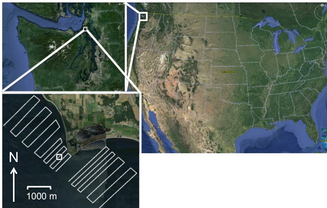
Figure 2.1. Admiralty Inlet, Puget Sound, USA. (top left) Admiralty Inlet at the mouth of Puget Sound. (bottom left) the location of the stationary echosounder, at a proposed tidal energy pilot site, is denoted by the white square in relation to the two spatial grids north and south of the stationary package, each consisting of high and low resolution transects.
